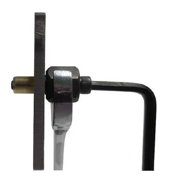
3. Break the nut loose by turning the hex nut wrench in a clockwise direction. Remove both wrenches from the tool. Remove tool from threaded insert by turning the cap head screw counter clockwise.
