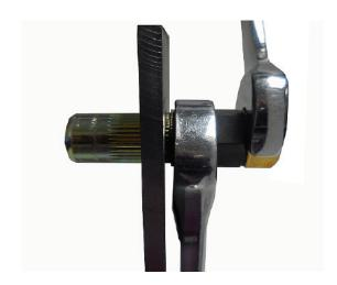
3. Break the nut loose by turning the wrench on the bolt in a counter-clockwise direction while using the other wrench to hold the tool body stationary.
